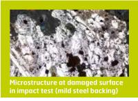
Under lab impact testing, the microstructure of the damaged surface of Duroxite™ 101 exhibits some plastic deformation, but the primary carbides are not worn significantly. It shows better impact resistance with the Hardox 450 backing plate compared to mild steel.
